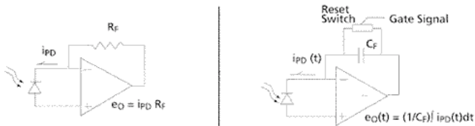
Figure 6b. Linear and Integrated Transimpedance Amplifiers
